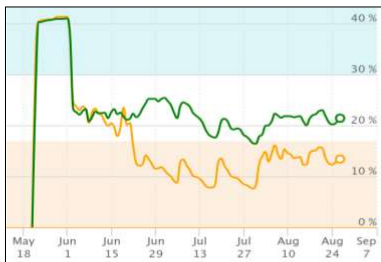
Figure 5. Volumetric water content recorded by Sensoterra probes at 15 cm (orange) and 30 cm (green) depths. The white shaded area represents the target soil moisture range between field capacity and maximum allowable depletion; green bars along the x-axis indicate 12.5 mm irrigation applications.
